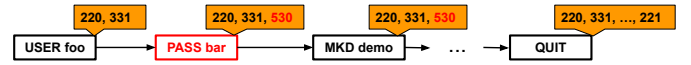
Fig. 6. A sample mutated sequence if the state 331 (User OK) and the message sequence in Figure 3 have been chosen.
